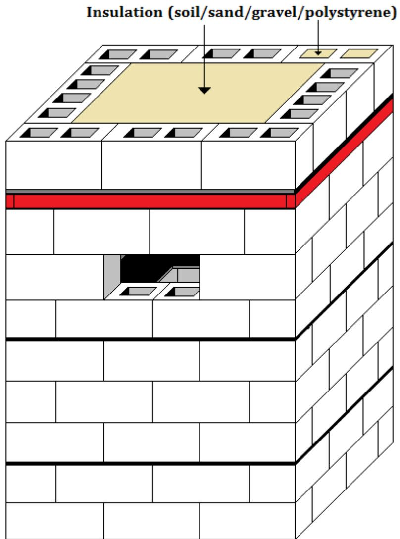
Fig 7. Tower with timber supported ceiling/roof and insulation
