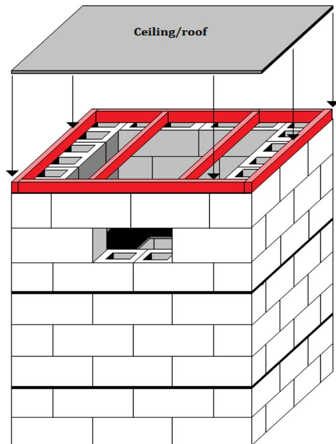
**Fig 6: Alternative roof/ceiling construction using 100 x 50mm timbers.**
